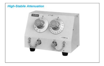
The MN95D optical variable attenuator passes an optical signal from a light emitting element through an optical fiber via a lens through an attenuating filter to reduce it to an appropriate light power output. It is a reflection type using metallic film and is used in the 1.3  $\mu m$  band. The MN95D can be varied continuously and in steps.
